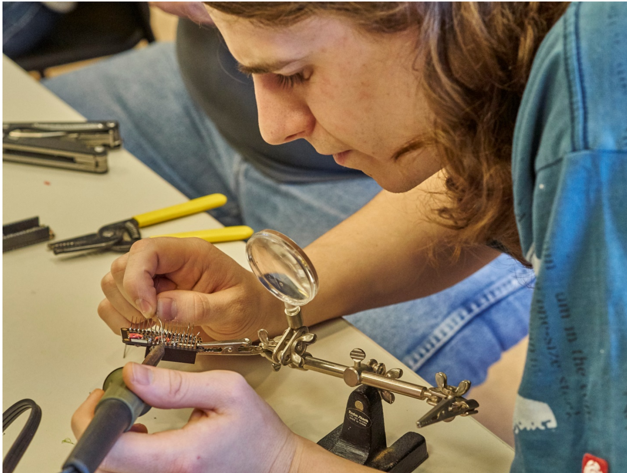
A Tompkins County 4-H member assembles a prototype LoRaWAN sensor module (Cooperative Extension, 2016)
