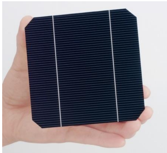
Figure 3: Typical size of a solar cell. These are what actually generate the electricity in a PV system, and a number of them are strung together to form a PV panel.
