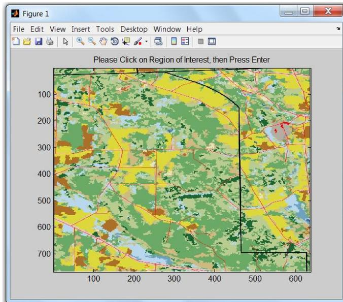
**Figure 2: Program User Interface. Program allows users to input an image and select the area of interest. The image must be color coded. In this case, brown represents land available for biomass harvesting. Green represents forests.**
