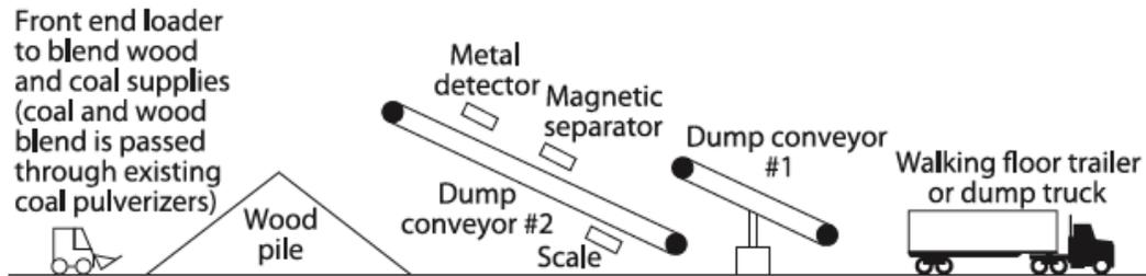
After the biomass product is delivered to the receiving bin, a hopper grinds it to a size comparable to that of pulverized coal.
